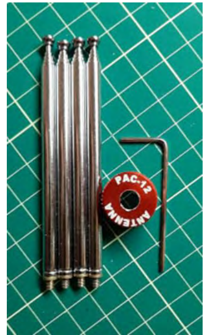
AliExpress top hat for a PAC-12 antenna. NB: I drilled a through hole in the hub to fit it on my tactical whip.
