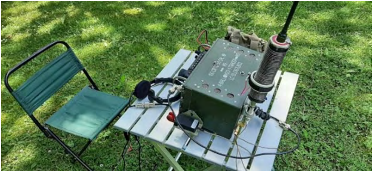
VA3KOT's trail-hardened FT-891 rig with ham-made adjustable loading coil and 9.5ft top-hat loaded whip
