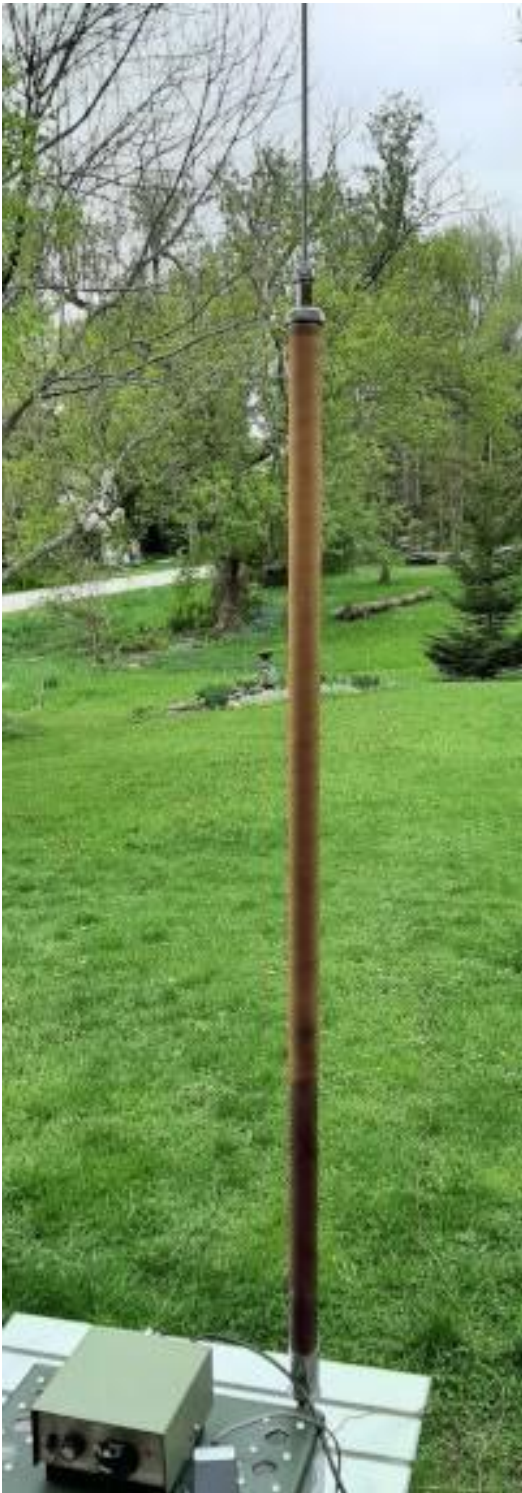
A Manual Screw Driver Antenna dating back to the 1950's.
