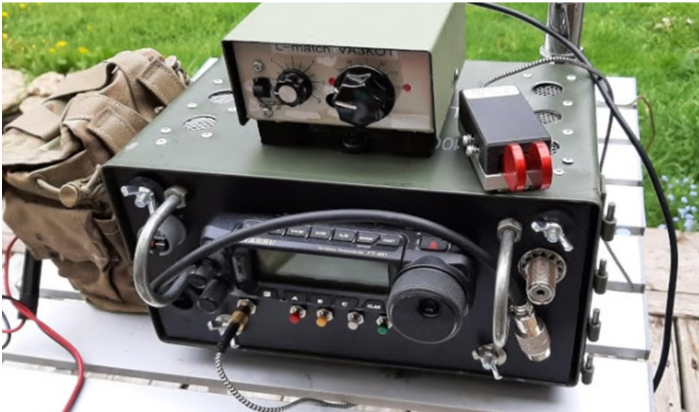
Ammo can radio set with FT-891 transceiver; ham-made L-match; CWMorse extruded aluminum paddles; Bioenno 12Ah LiFePO4 battery in canvas pouch (left of picture) and Webster Band Spanner antenna attached at rear.
