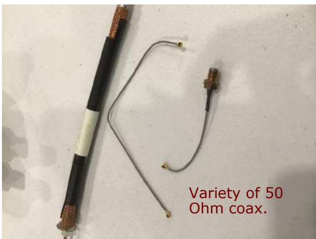
A cornucopia of various feedlines, common coax and hardline including a huge array of connectors for various types.
