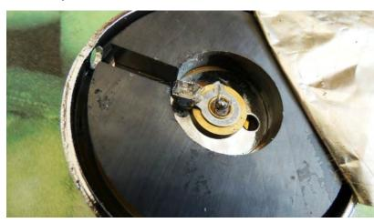
As you can see from the picture in the left, there are two points to solder: the inner part of the cable, and its ground.
