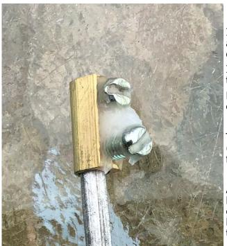
I slid the barrel over the end of the antenna tip and replaced the screws and tightened the barrel onto the antenna. Again see the picture.
