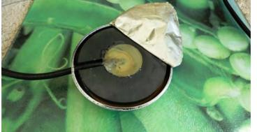
net and the cable. I flooded the cable part with the wax and I added glue on the magnet and edges, for resealing. I also flooded the hole for the cable with glue.
