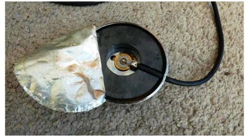
The base has a glued folio where it touches the magnet on one side, and a non-glued part to the exterior, that side that will touch the surface on which the mount will be attached to.
