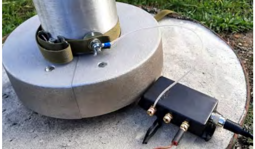
Connecting the base of the flagpole to the 4:1 unun (black box)
