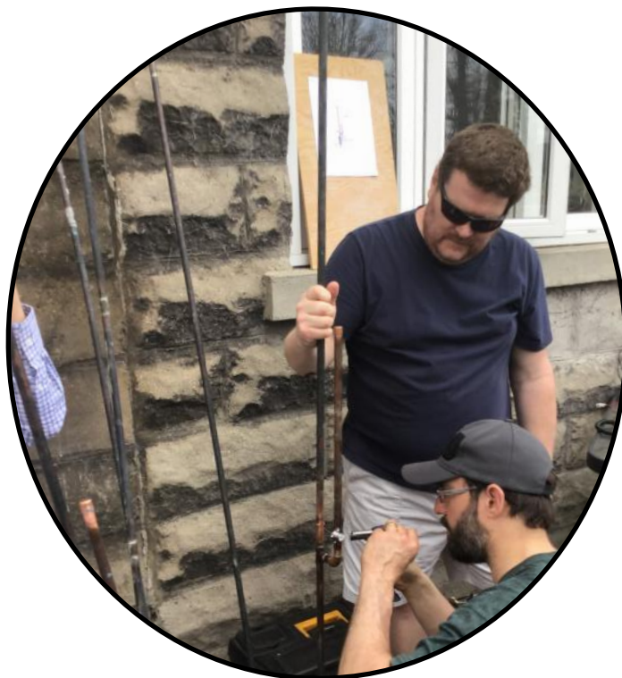
Brendan VA3BVB soldering an SO-239 connector while Dwayne VE3CQQ holds the J-Pole steady.
