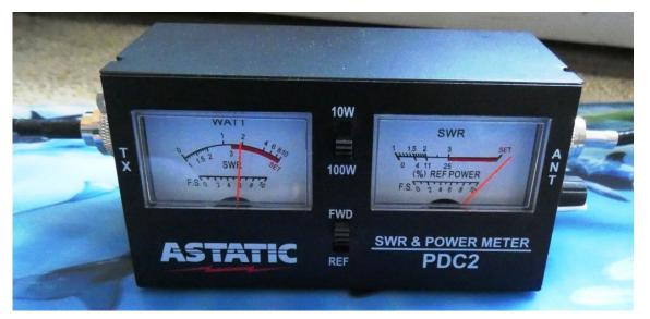
The right side potentiometer must now be rotated until the indicator on the right meter is at the maximum of the red zone, where the meter indicates SET. My transmitter generates 20 Watts towards the antenna (see left meter), so I required the 100 W scale range. If the indicator is very low, just move the slider into the 10 W position, and re-adjust the potentiometer to move the needle to SET, at the end of the red zone, in the right meter.
