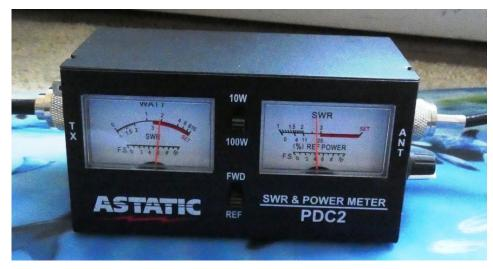
Move the lower slider into the REF (reflected) position. Transmit again. Now we can read the SWR on the right meter. As you can see my antenna is not great at 3. (I used a 2 meter transceiver, with a different antenna not designed for 2 meter).
