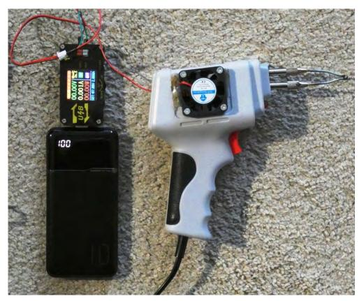
I had a variable power adapter and I started to solder, to see if the experiment worked. The transformer did not overheat anymore. The soldering gun now cools itself. Some 5 – 6 Volts are enough for efficient cooling. The next step is to disassemble the soldering gun again, make the plastic sealing nice and add a switching power supply small board inside the handle as I can find plenty online with \$3 – 4 CAD, drawing under 300 mA.
