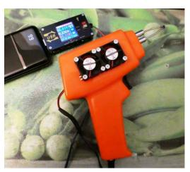
The consumption for the two 3010 fans, at 5V is 230 mA. The orange case is more generous with space, and it is easy to install a small switching power supply board for the fans inside the handle. The result was good and ready for a test. I had some connectors to solder, some transistors to take out from an old board, and a piezo filter before I finally stopped. It worked perfectly. Because it is under 500 grams, the whole soldering gun with the fans is very comfortable to handle.
