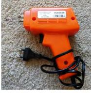
The gray one has more cooling vents than the orange model. The tip is directly held by two screws for the orange model. The gray model has a kind of flower with 4 petals into which the soldering tips are inserted, and screw caps on top of the flower keep everything tied. Both soldering guns are low quality. They overheat and the gray model easily breaks the soldering tip catching parts. So
