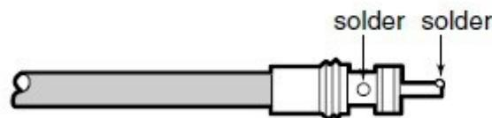
③ Slide the connector body on and solder it.
