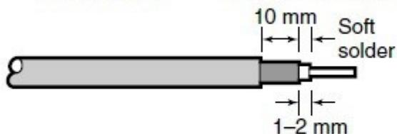
② Strip the cable as shown at left. Soft solder the center conductor.
