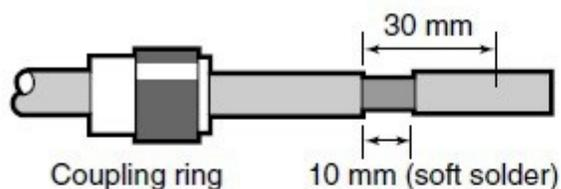
① Slide the coupling ring down. Strip the cable jacket and soft solder.
