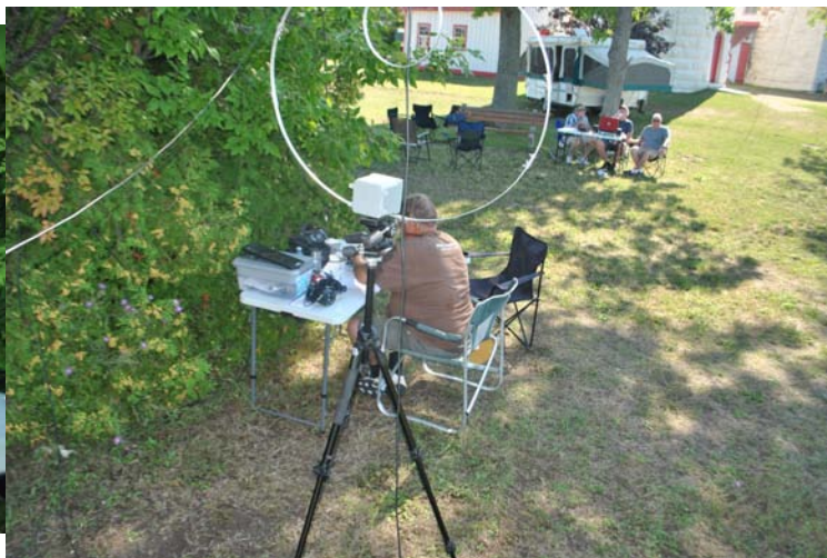
Ken VE3KCY working 40 M CW with his magnetic Loop antenna. With his very first call he logged an Iowa station.
