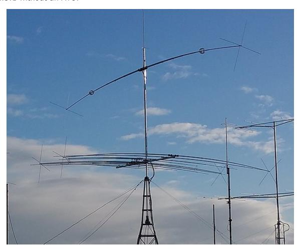
So how has this been done? Many hams and antenna companies have made the mistake of installing low efficiency coils far too close to the dipole centre. The Delta C-140 uses a combination of capacity loading and large diameter coils moved out much further out either side of
