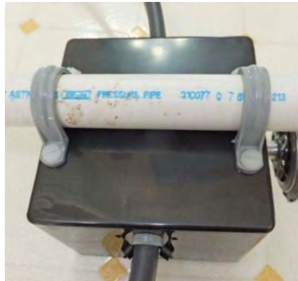
The plastic clamps (and the capacitor) are attached with 1/2" x 3/16" nylon bolts.
