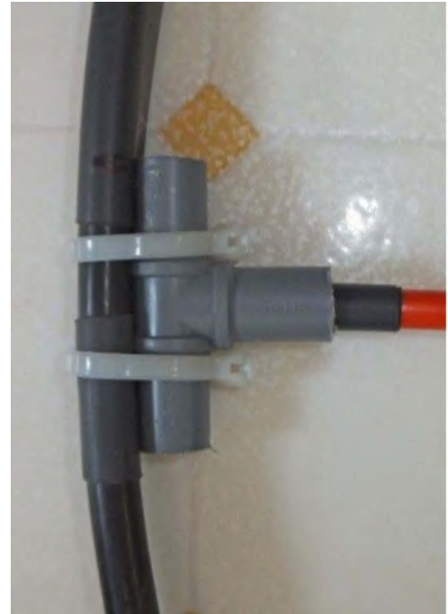
A hose tee with shortened arms is used to secure the loop to the support arm.
