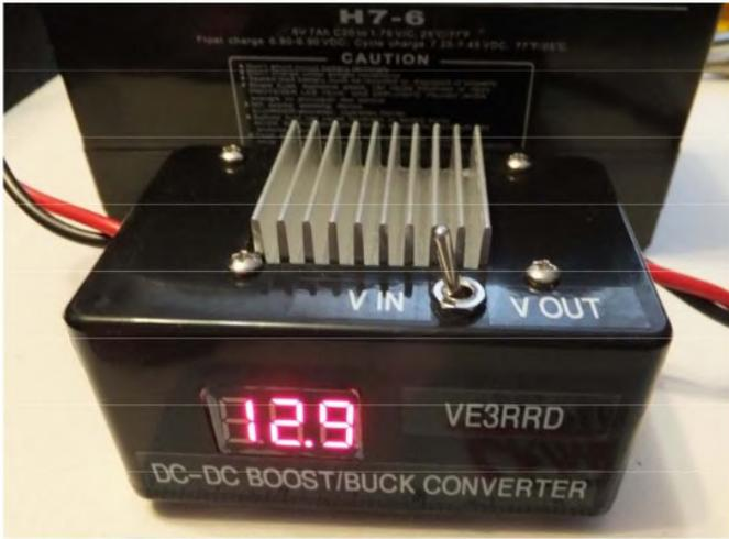
This voltmeter is powered by the voltage it is measuring, and operates over a range of 2.5 to 30VDC. The finished converter allows me to use 6V, 12V or even 24V batteries to power my KX3
