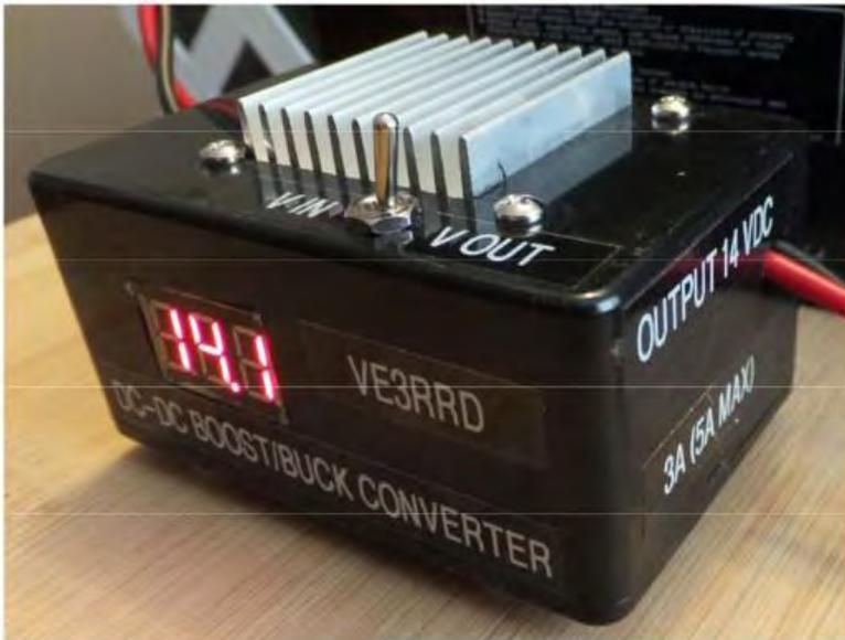
or the output voltage. The KX3 has a series diode in the power supply line, so I adjusted the converter output voltage to obtain the desired voltage as displayed on my KX3. An output of 14.1V resulted in a displayed value of 13.9V on my KX3. I used 18 AWG wire for both the input and output cabling to minimize voltage drop. At maximum output current and lower input voltages, the converter can draw as much as 8A intermittently from the battery.
