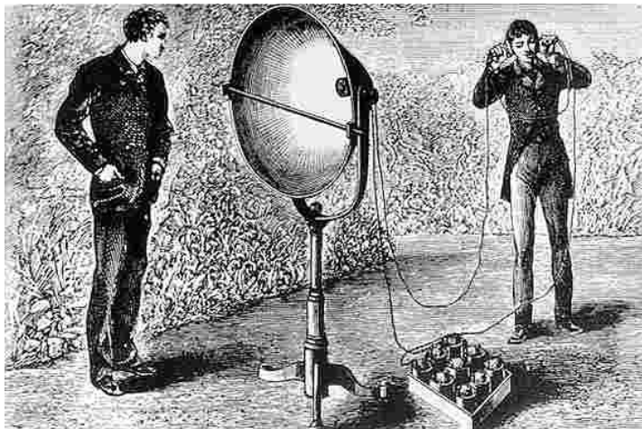
Photophone receiver, one half of Bell's wireless optical communication system, ca. 1880
