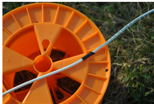
The spool coiled dipole above. Shown below are the markings to indicate the wire lengths.
