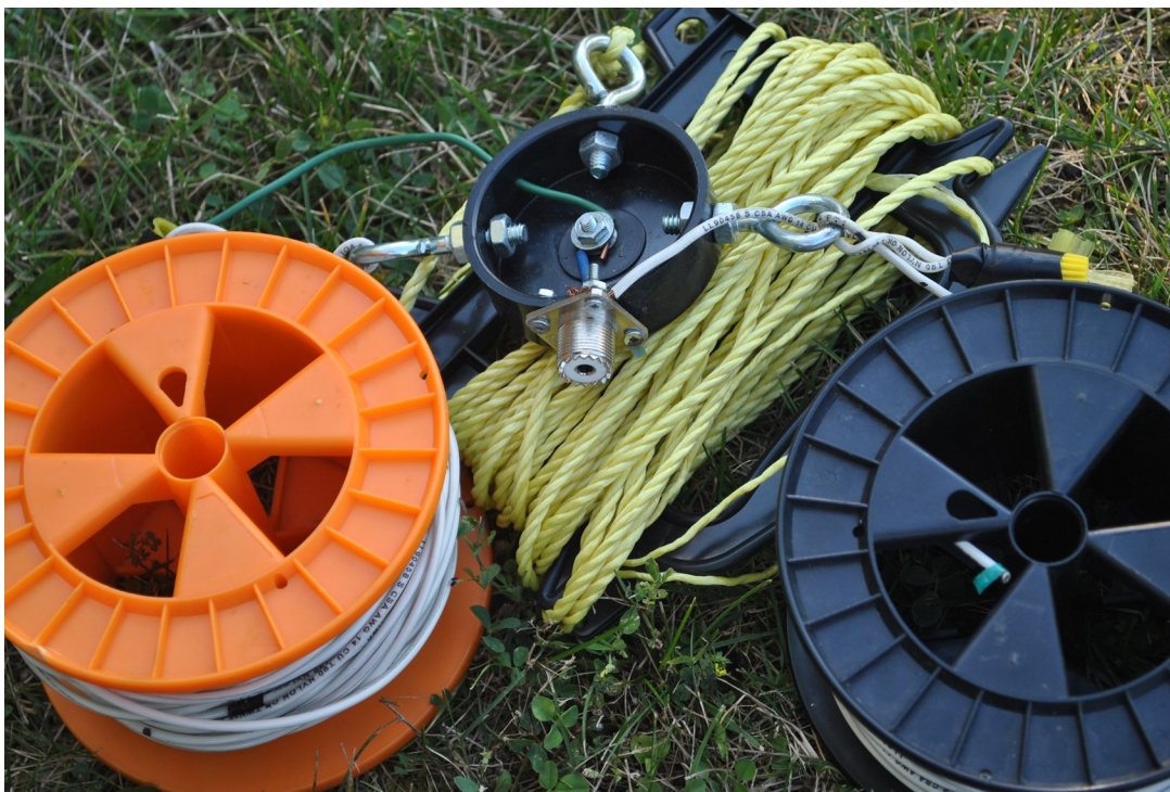
The spool coiled dipole above. Shown below are the markings to indicate the wire lengths.
